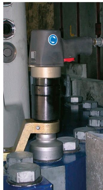
alkitronic® PC-S torque multipliers in use (figures on the right). Screw connections at a bolt circle and a diesel unit for large construction machines
